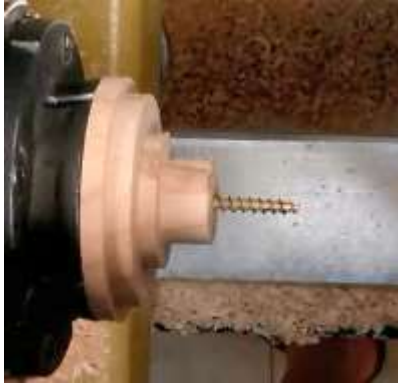
Figure 7 Spigot that fits the inside of the mill head.
