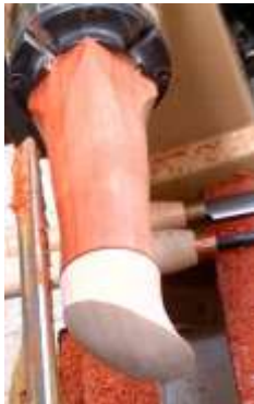
Figure 9 Shape the top of the mill body with the bottom secured in the chuck.
