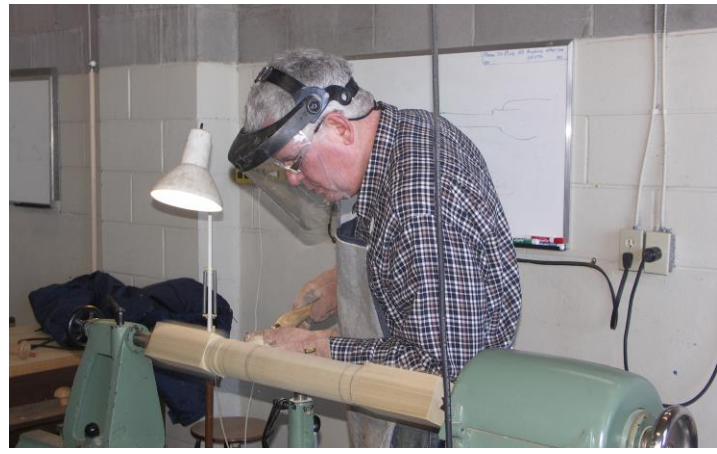
The various pattern sections have been marked with pencil on the rounded post, ready for turning.
