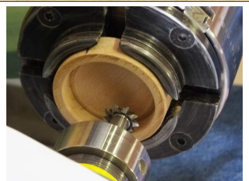
The 16 TPI cutter is positioned ready to begin the threading cut on the lid.
