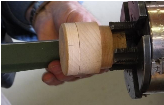
Lid screwed onto the box base to shape the outer box profile.
