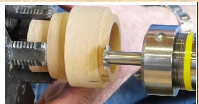
Cutter positioned to do an outer cut on the lip of the box base.
