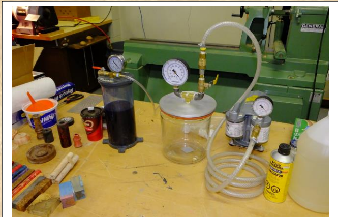
Dave's glass vacuum chambers for "soaking" the samples.
