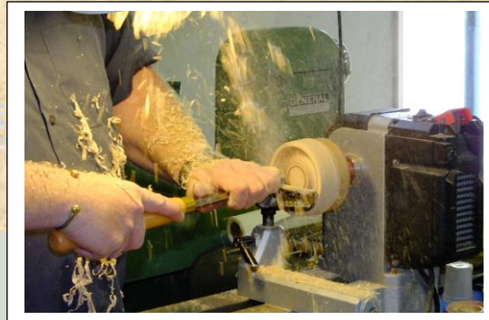
Shaping the inside of the call, using the 1/2" round nosed scraper.
