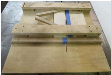
The width of the linear staves is adjusted by screws in the 2 slots of the **Width Stop**. The blank is fed along the **Back Stop** from the left side and butted against the **Width Stop**. Two long slender tapered wedges were used to secure the blank being cut; one under the **Front Bridge**, one under the **Back Bridge**.
