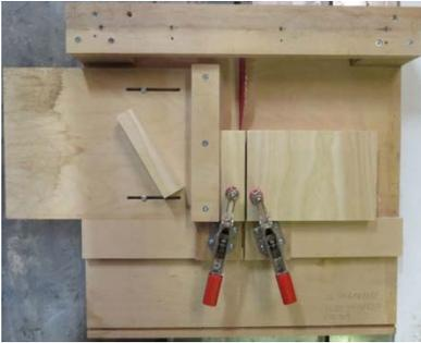
The **Linear-Stave Cutting Jig** in the **Linear-Stave Vessel** presentation is a simple homemade fixture to securely hold pieces of wood from which to cut linear staves using a table saw. The wide side of the linear stave being cut was oriented up to provide ample clamping surface for a hold-down clamp.
