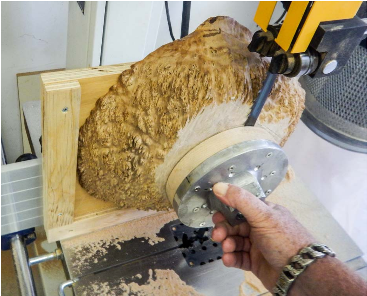
Step 6... cut off sacrificial block using bandsaw
