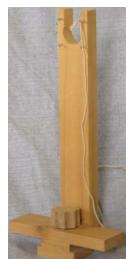
centre of the lathe. As shown in the picture of the bedway-mounted string steady rest, attach the base of the upright to a cross member which sits on top of the bedway. Attach a thin block, which is the width of the bedway gap, centered on the bottom of the cross member. Make a clamp block, which fastens to the string steady rest cross member from under the bedway, typically by a bolt and nut.
