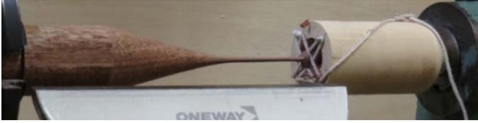
A tailstock mounted (MT1, MT2, or MT3) string steady is a simple homemade lathe accessory to steady long thin turnings on the lathe. With the string steady mounted in the tailstock, move the tail stock toward the
