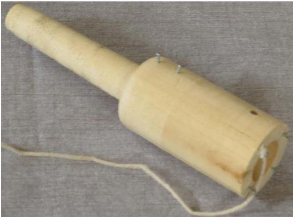
Practically any scrap wood, of appropriate dimensions, can be used, for example, a scarp piece of 2X2 construction spruce. Turning blank should be at least 1 1/2" square and at least 6 1/2" in length.
